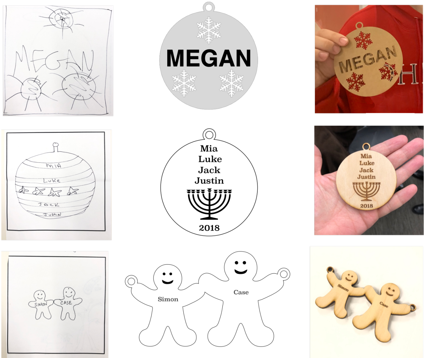
Figure 3: Each row above represents the three stages of a particular participant’s design process. On the left is the sketch each participant created for reference; in the middle is the design as created by the design wizard; on the right is the final fabricated ornament for each participant.
